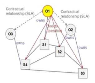
Figure 7: SoS and Constituent System Relationships in an Acknowledged SoS<sup>18</sup>.
